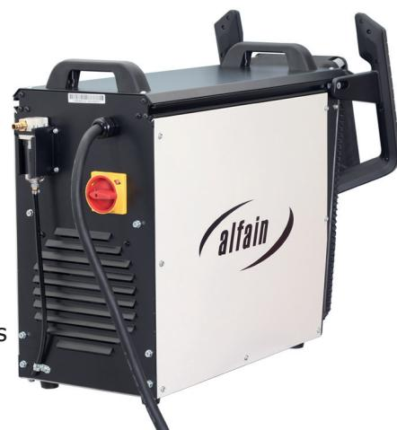
SVAROG 105 PLASMA is designed for high-quality cutting of materials up to 45 mm thick carbon steel. Productive cutting of carbon steel can be to the thickness of 22 mm. At lower demands on the quality of the cut can be cut through (separate) the material thickness to 50 mm.
