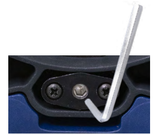
Unlock or lock a battery using an inbus key
