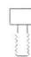
(9-65XX) 3/16" Capscrew (3/8" Long) (Used on bush & roller guide when # 9-6515 adapter sleeve is in place)
